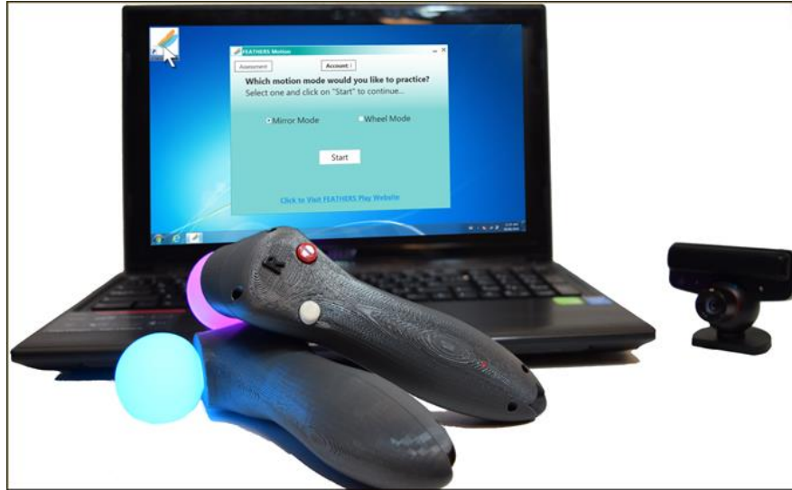
Figure 1. FEATHERS System. Included: laptop computer, a PlayStation Move camera, and two ergonomically modified PlayStation Move wireless hand-held controllers.
